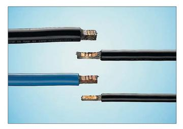
In addition to welding tinned wires together, the Sonobond SonoWeld<sup>®</sup> and Sonobond SpliceRite<sup>™</sup> ultrasonic metal welders are used to weld tinned wire to tinned terminals as well as to bare and coated wires and terminals.
